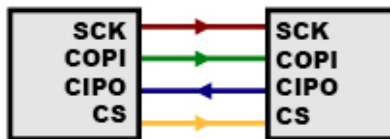
Fig. 17: Controller-Peripheral SPI configuration 1 to 1
