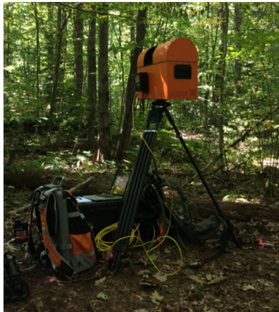
Fig. 7: DWEL dual wavelength laser.
